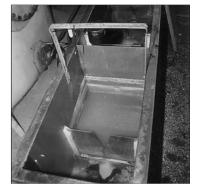
Measuring box supplied for wastewater outlet at dairy. With the little flow that is measured it is best to use a prefabricated measuring box where the 90° weir is mounted directly on the measuring box.
